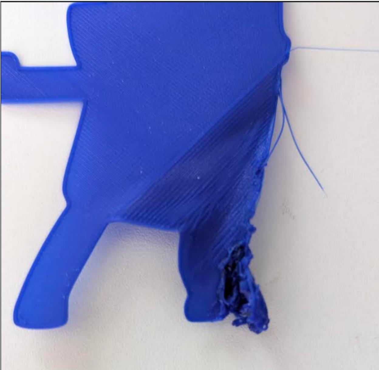
The solution seems to be to slow down the initial layer. From 50mm/s to 30mm/s
